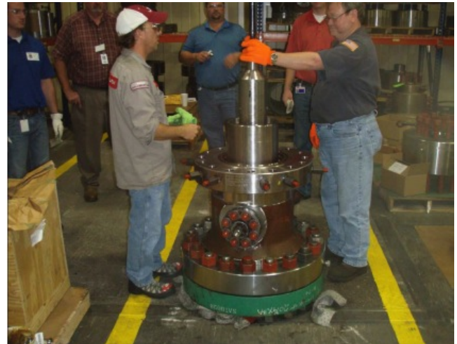
Figure 11 – Stack-up Test of Tubing Hanger and BPV
